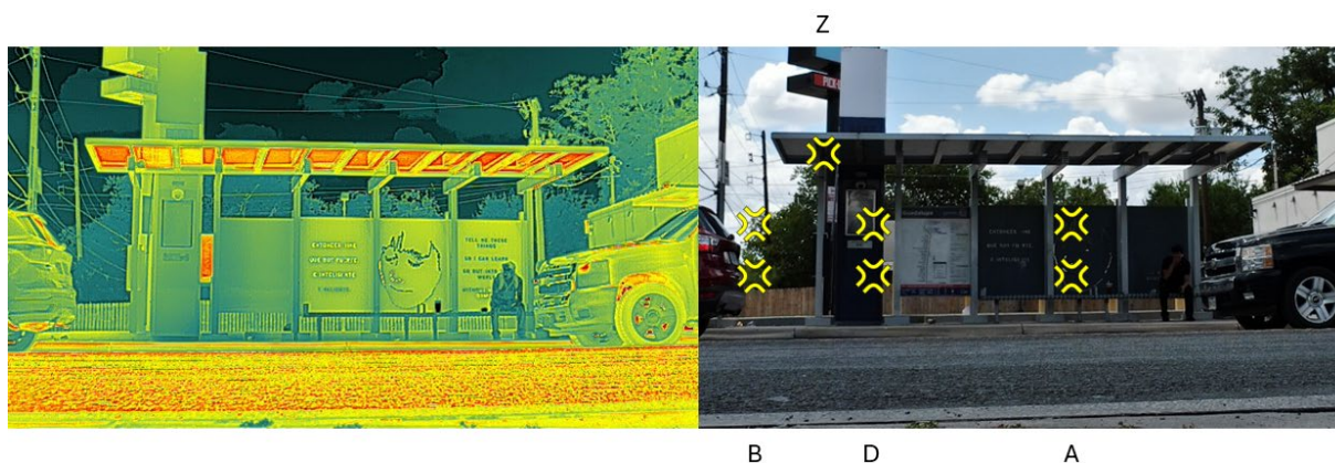
Figure 15. Thermal and visual imaging of Bus Stop 21607, one of the Primo stations, on August 6, 2025, with the Kestrel monitoring sites noted.
